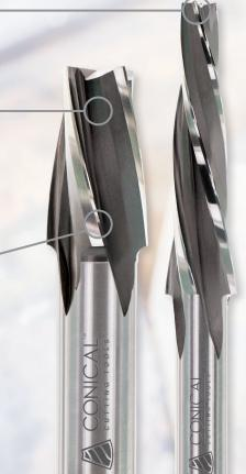
No end cut to increase tool stability and edge strength
