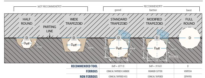
Above are common cross section designs for runners. The last three designs are generally recommended and each have unique properties which add pros and cons to their use.
